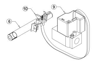
Figure 11.3a: Gas Valve and Pilot – Standing Pilot (Continuous Ignition)
